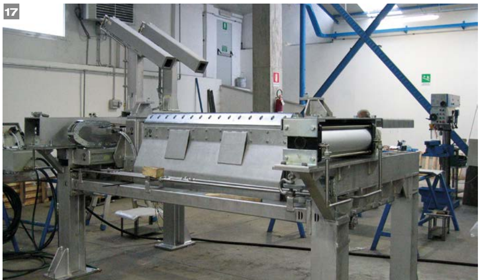
14-17 Deburring machine for slabs 15 Deburring machine for 600 rounds 16 Deburring machine for blooms
